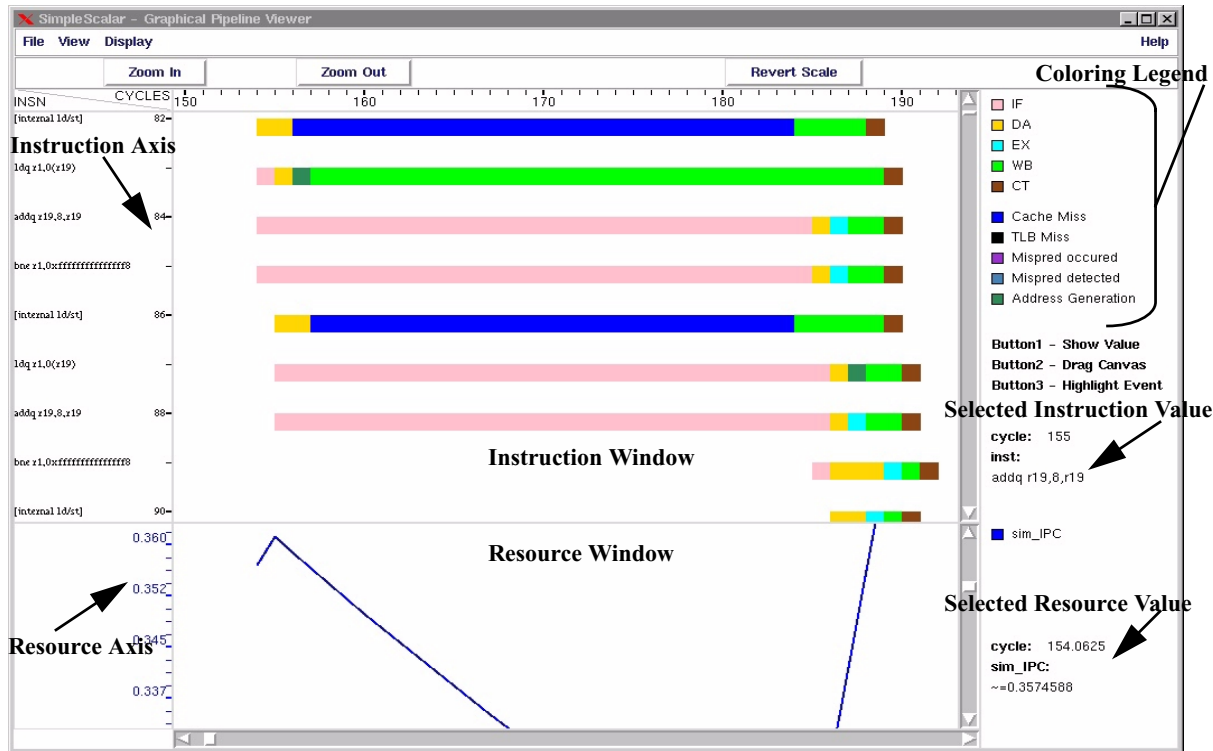
Figure 2: GPV Display Window. This example shows the execution of instructions on a 4-wide Alpha ISA model. (Note: Internal micro-code operations, i.e. internal ld/st, are allowed to finish out of program order.)
